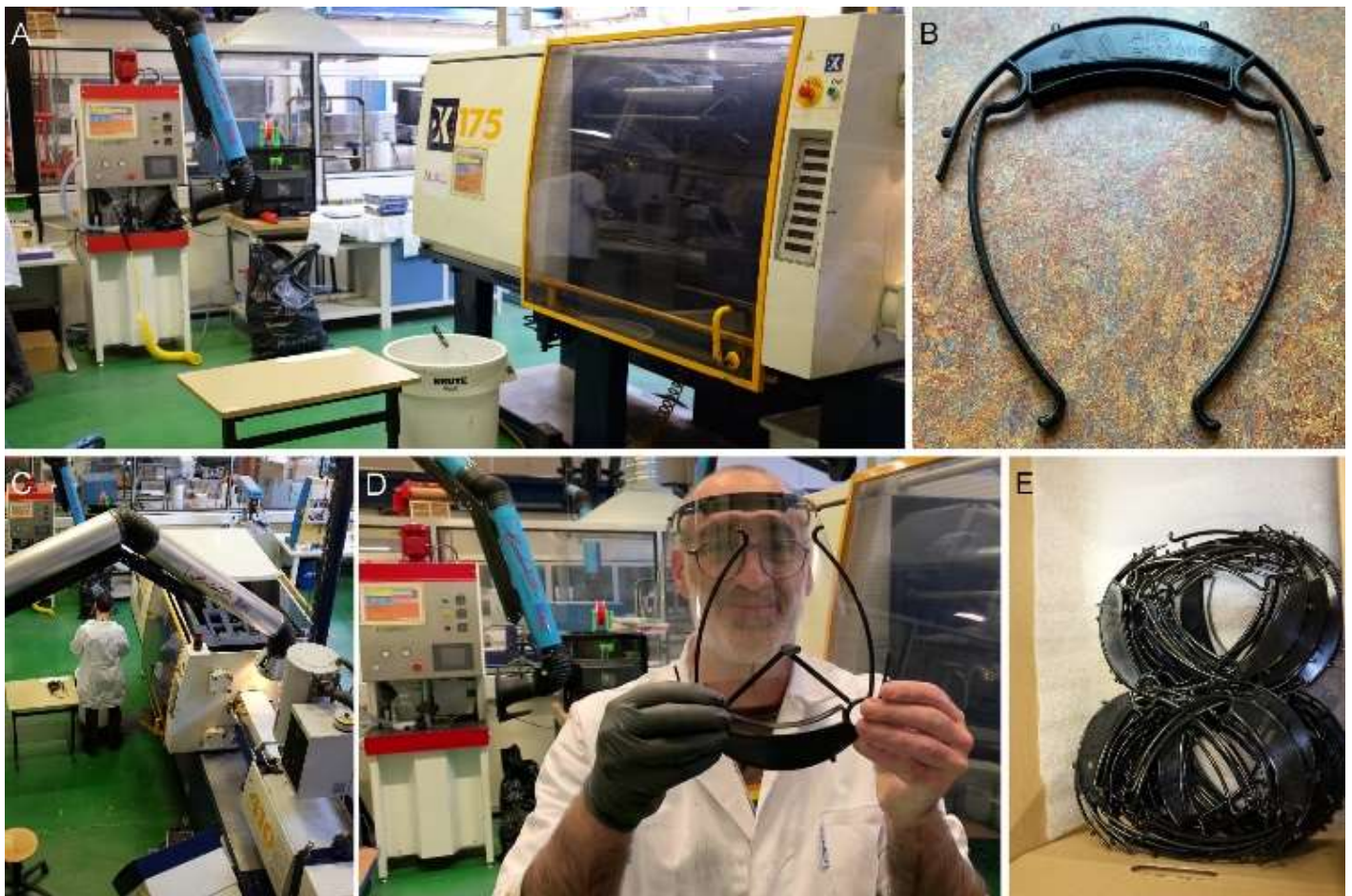
Figure 9 : Production at the laboratory. A Injection press of the PIMM. B Head band injected in polyamide 6. C- production session. D- Face shield in use. E- hourly production of head-hand
