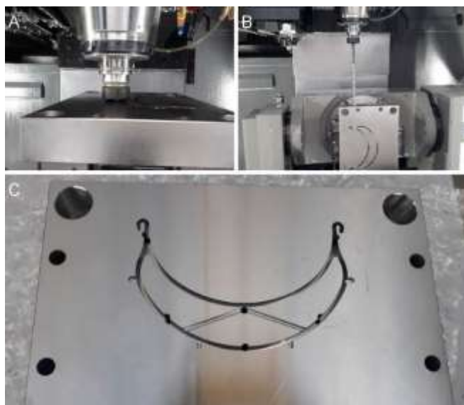
Figure 3 : Mold imprint fabricated at the Arts et Métiers campus of Bordeaux. A, B : machining steps. C: final imprint for injection
